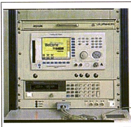
3. CDMAOne test stations should incorporate minimum hardware to support focused testing of only the manufacturing process.
