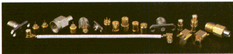
Shown at actual size, K and SMP ("GPO" compatible) connectors frequently used in OC-192 equipment.
