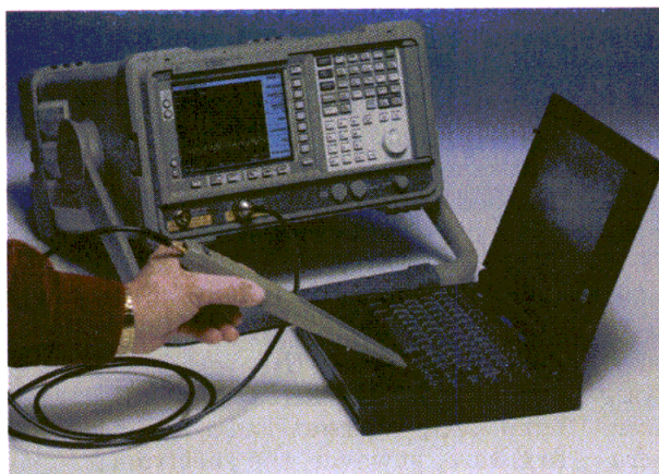
2. The EMI receiver or spectrum analyzer is a critical part of an EMI precompliance test system.
