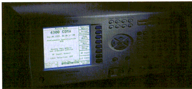
4. The WWG MMS-4300 will incorporate a CDMAOne codec in the future to facilitate audio testing.
